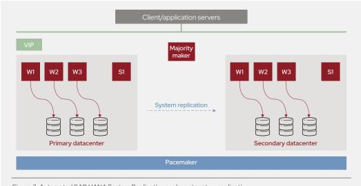
Figure 3. Automated SAP HANA System Replication scale-out system replication.
